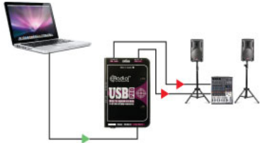
Using the USB-Pro with a laptop
