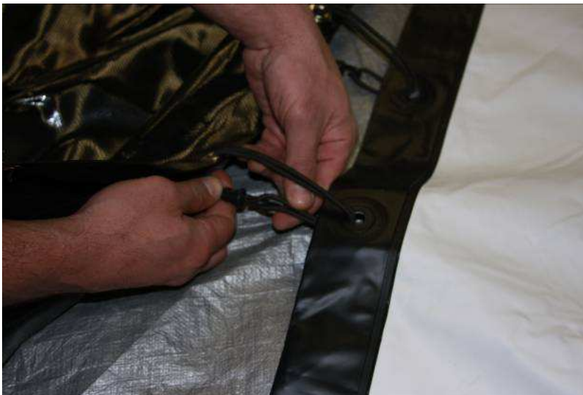
image 12 - Clip looped end of bungee to bungee clip
