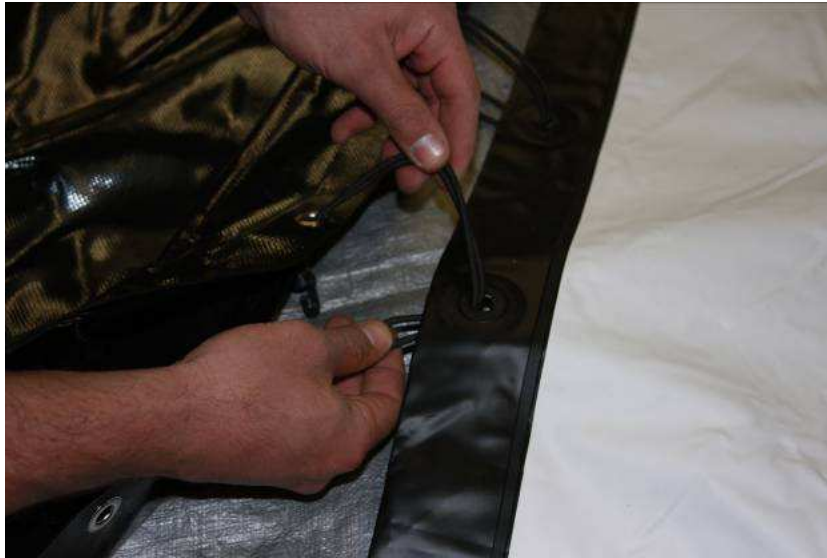
image 11 - Bring end of tie through the screen grommet from front to back
