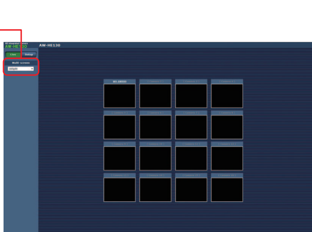
Multi screen consisting of 16 sub-screens
