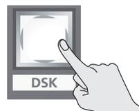
The [DSK] button lights up in red, and the text or image is composited and the results are output.
