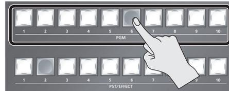
2. Press a cross-point button in the PST/EFFECT section to select the video to overlay.
