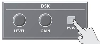
The DSK [PVW] button lights up in green, and a preview of the composition results is displayed in the PVW section of the multi-view monitor.
