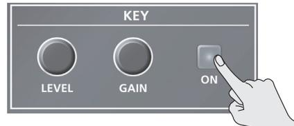
The KEY [ON] button lights up in green, and a preview of the composition results is displayed in the PVW section of the multi-view monitor.
