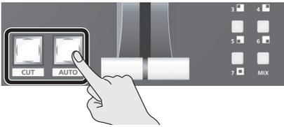
The video you selected in steps 1 and 2 is composited and output. At this time, the KEY [ON] button and the cross-point button in the PST/EFFECT section light up in red.
