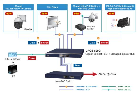
With data and Power over Ethernet from one unit, the UPOE-800G can reduce power cable deployment and eliminate the need for dedicated electrical outlets on the wall, ceiling or any unreachable place.
