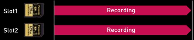
Identical data is recorded onto cards in both slots in this redundant recording mode.
