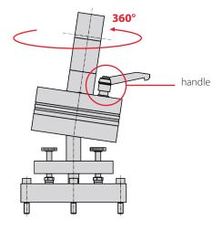
When turning the handle on the truss mount, it becomes mobile and can be rotated by 360°.
