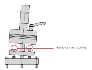
By means of the 4 adjustment screws, the positon of the mount can be defined very precisely.
