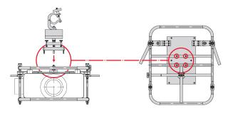
Place the truss mount on the rear side of the frame. Make sure that the 4 screws enter the 4 holes in the frame. Tighten the screws to secure the truss mount on the frame.
