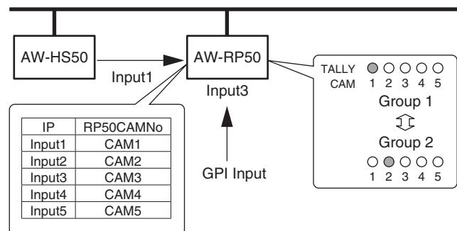
In response to inputs 1 to 5 from GPI Input, tally indicators CAM1 to CAM5 are lit in red, and the tally ON instruction is sent to the remote cameras concerned.
