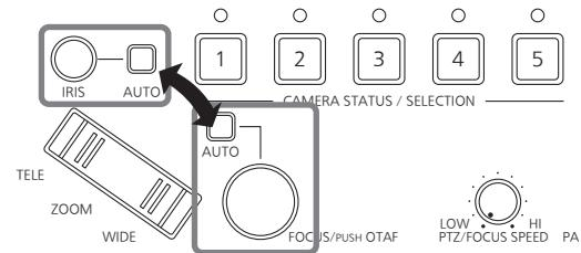
From the [SETUP] menu, select [OPERATE] and display [FOCUS/IRIS]. Then select either "STANDARD" or "EXCHANGE".
