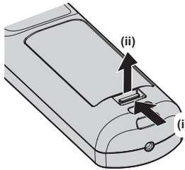
**2. Remove the batteries.**
