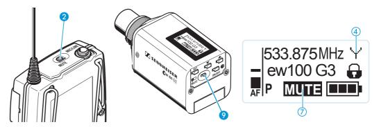
The MUTE switch ② (SK)/ ② (SKP) allows you to mute the audio signal or to deactivate the RF signal. Via the "Mute Mode" menu item, you can set the desired function of the MUTE switch ② (SK)/ ③ (SKP):
