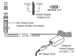
**CAUTION:** This product is intended to be supplied by a Listed Power Unit marked "Class 2" or "LPS", rated 12 VDC, maximum 1.0 A. Always use a power supply supplied or specified by Extron. Use of an unauthorized power supply voids all regulatory compliance certification and may cause damage to the supply and the end product.
