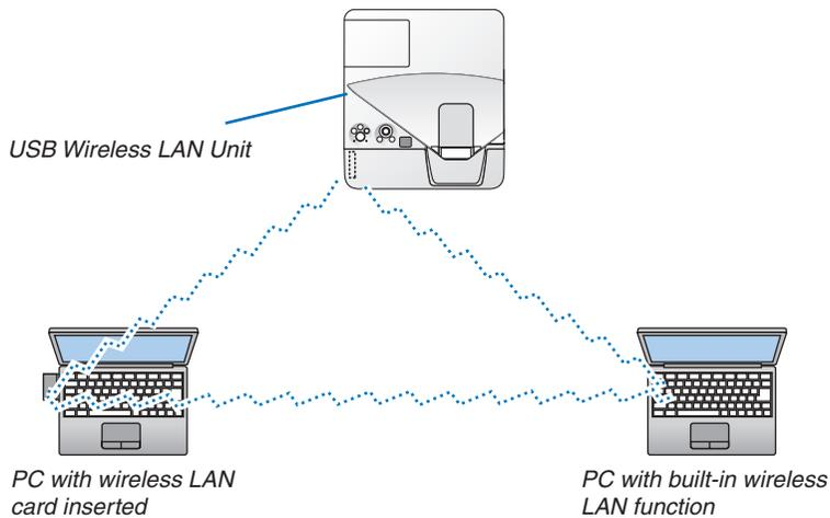
To enable direct communication (i.e., peer-to-peer) between personal computers and projectors, you need to select the Ad Hoc mode.
