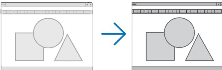
**PHASE**..... Use this item to adjust the clock phase or to reduce video noise, dot interference or cross talk. (This is evident when part of your image appears to be shimmering.)
