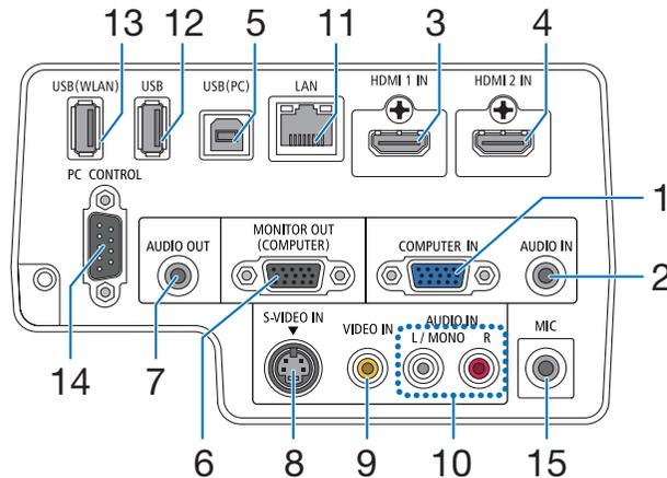
1. **COMPUTER IN/ Component Input Connector (Mini D-Sub 15 Pin)** (→ page [106](#), [110](#))
