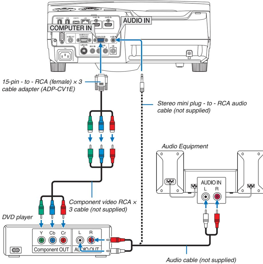
A component signal will be automatically displayed. If not, from the menu, select [SETUP] → [OPTIONS(1)] → [SIGNAL SELECT] → [COMPUTER], and then place a check mark in the Component radio button.
