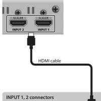
These input video. Connect these to a video camera, video device such as a BD player, or a computer that is equipped with an HDMI output connector.
