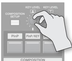
\* Turning this knob also changes the value of the Key Level setting at the PinP/KEY setting screen.
