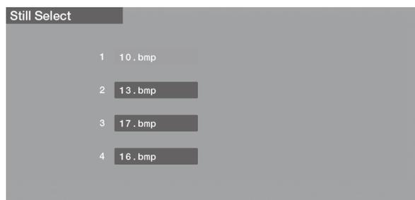
**3. Touch the name of the file, then press the VIDEO INPUT SELECT [STILL] button, making the button's indicator light up.**
