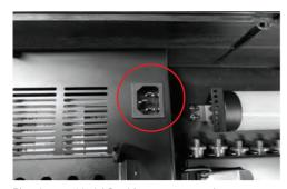
Plug the provided AC cable to power supply.
