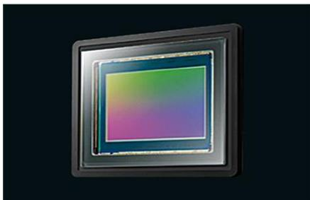
The 1.0-type MOS (approximately 15,030,000 pixels) offers an outstanding depth of field and excellent balance between image quality and sensitivity. It supports multi-formats, such as UHD (3840 x 2160), FHD, HD and SD, and provides images without cropping in all modes. This MOS sensor also boasts high sensitivity of F12 (60 Hz) /F13 (50 Hz) (in both UHD and FHD in High Sensitivity mode).
