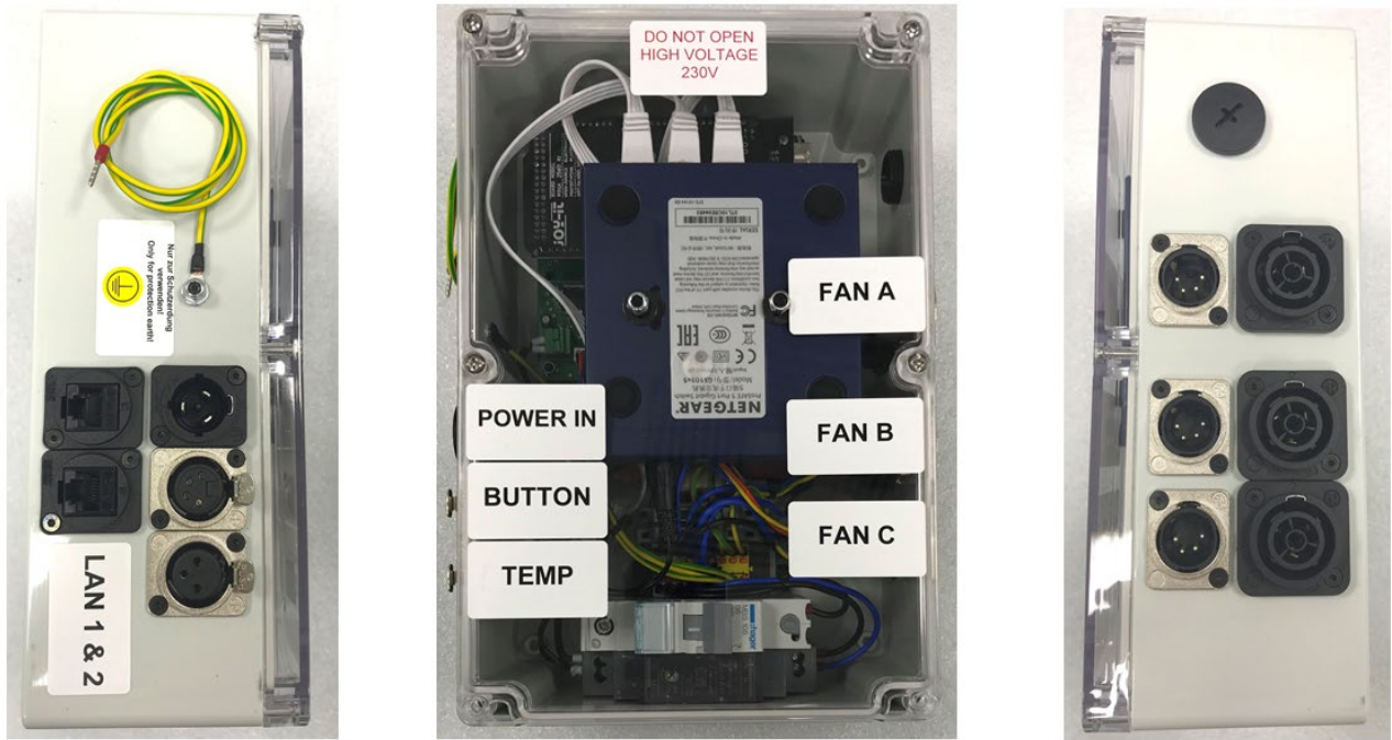
Figure 18 CU with connections on the sides
