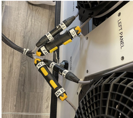
Figure 31: Connection of FAN B and FAN C
