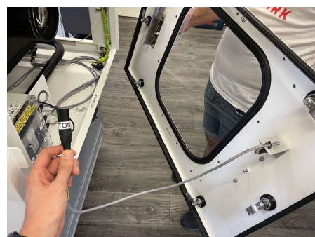
Figure 10 Installation of Front-Panel and connection of the button
