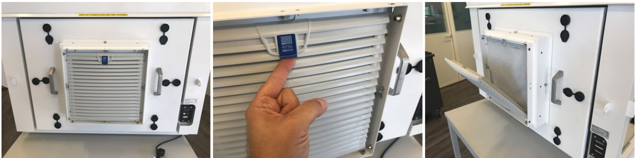
Figure 24 Installation of filter air outtake
