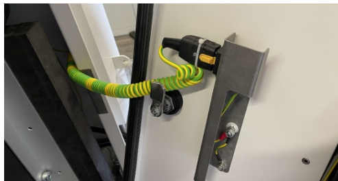
Figure 25: Connection of the grounding to the Rear Panel
