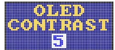
The display contrast is adjusted to its maximum intensity, and if the beltpack remain quiet for thirty seconds, the display contrast level will fall, and if remain quiet for another thirty seconds, the display shut off automatically, turning on when any key, or an external event occurs.
