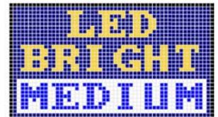
The LED bright is adjusted to its maximum intensity, and if the beltpack remain quiet for thirty seconds, the LED bright will fall to medium level (if it is adjusted to high level), and if remain quiet for another thirty seconds, the LED bright will fall to low level (if it is adjusted to medium or high levels), turning to the level adjusted when any key, or an external event occurs.
