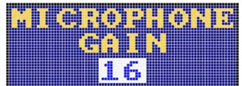
The microphone gain can be adjust directly (without menu), pressing the MIC ON/OFF
