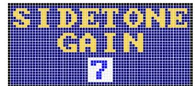
The SIDETONE GAIN, it is stored in the unit. Press again to switch on the buzzer.
