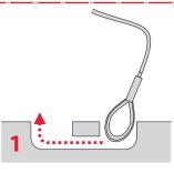
Please use the enclosed steel wire to secure the projector in the frame by drawing the wire around the securing bar (1) of the projector as shown in image 1.
