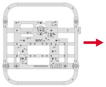
Place the frame on the projector so that it is aligned with the screw hole positions. (Make sure that the forward/back direction is correct when installing. If the direction is reversed, the hole positions will not match.)
