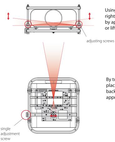
Using the adjusting screws to the left and right you can adjust the position of the projector by approximately five degrees. You can lower or lift the front left or right corner.
