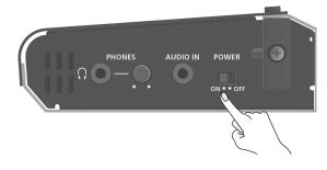
3. Turn on the power in the order of source devices → output devices.
