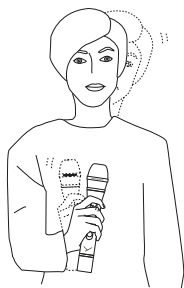
How to hold the microphone when using the “Far” setting
