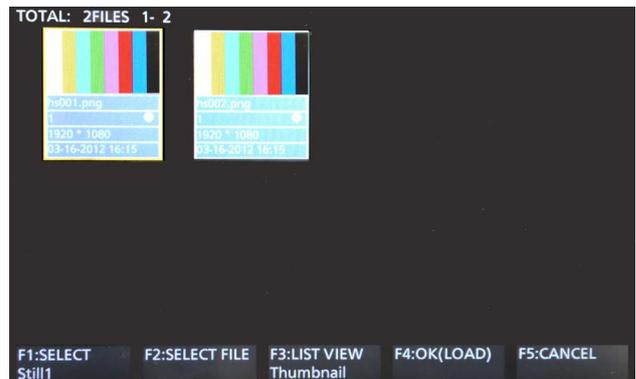
For Still thumbnails, the image is displayed in the upper portion, and the file name, KEY indicator, image size, and file date are displayed in the lower portion.
