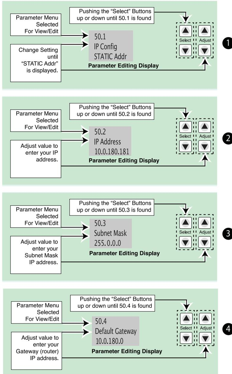
**Note:** for parameters 50.2, 50.3, and 50.4, you will be setting IP addresses that consist of "octets" separated by a period (i.e., 10.0.180.0).
